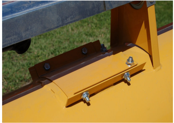
Fig. 31 BEARING REPLACEMENT (Access Covers)
